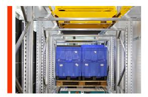
Integrated systems aim to minimize human touches by seamlessly transferring products between automated storage (such as ASRS) and processing stations (such as pick-andpack stations), reducing handling time and error rates.
